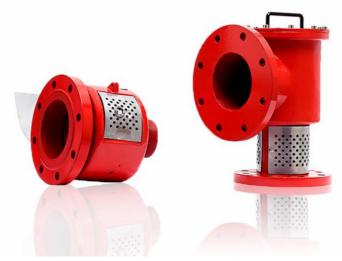
Air foam chamber is a fire extinguishing equipment fixed on the oil tank to produce and spray air foam to extinguish oil fires. Its foam proportional mixing device uses the foam mixture supplied by a fixed fire pump to flow through the pipeline to produce a certain pressure, and the foam formed in contact with air can extinguish oil fires.
