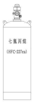
The bottle part is composed of steel cylinder and cylinder valve
