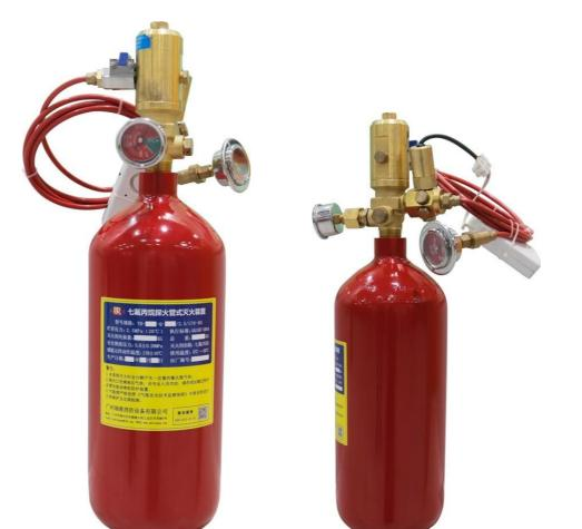
Fire Detection Tube is a reliable and cost-effective automatic fire detection and suppression system that installs in small enclosures or inaccessible areas. It actuates by a pressurized detection tube that ruptures when exposed to the heat and flame of the growing fire. The system requires no electricity and is easy to install and maintain. It is compatible with HFC-227ea or Co2, and direct release or indirect release systems are available.
